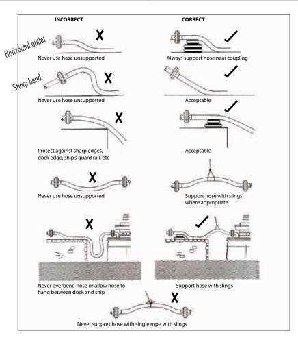
Use a **BEND RESTRICTOR** to prolong hose life when hose is used on horizontal outlets or sharp bends. (See also page 6) **Note:** Due to the inherent nature of composite hose it is susceptible to stretching in length while pressurized. Hose elongation while under pressure is not an indication of failure of films and fabrics. It is therefore critical that this be taken into consideration when calculating the overall length for a hose assembly in operation.
